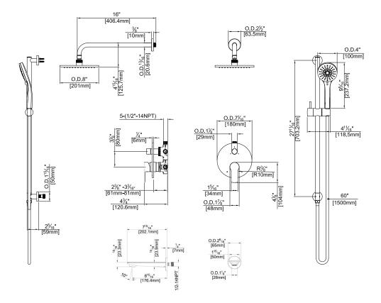
$\textbf{Codes and Standards:} \ \, \text{ANSI/ASME A} 112.18.1, \ \, \text{CSAB} 125.1, \ \, \text{IAPMO/cUPC Listed}, \ \, \text{EPA Watersense Listed}, \ \, \text{ADA Compliant}$
