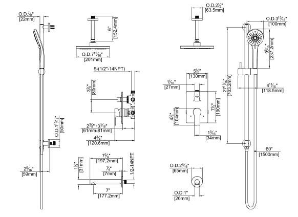
Codes and Standards: ANSI/ASME A112.18.1, CSA B125.1, IAPMO / cUPC Listed, EPA Watersense Listed, ADA Compliant
