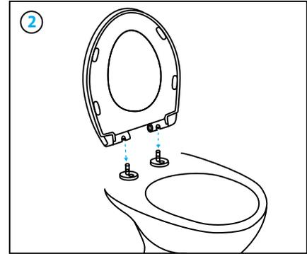
Insert hinge pins into the seat.
