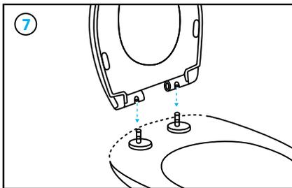
To clip the seat back onto mounting bracket, place the seat over the pins and push the seat downwards.
