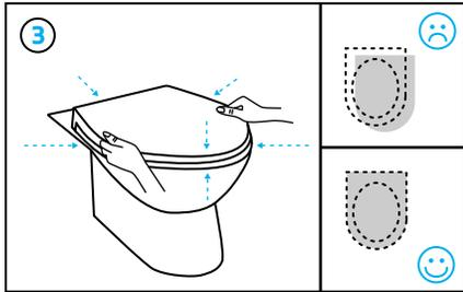
Close the seat cover, (do not force it closed). Straighten the seat front and edges to align with the edges of the bowl.
