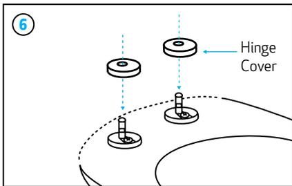
Remove any protective film on the hinge covers and place them over the hinge pin to cover the hinge.
