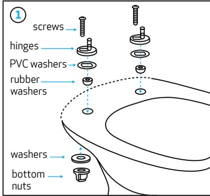
Insert component parts into the ceramic holes on your toilet bowl in the order shown order. Fasten from the bottom of the bowl. Do not fasten the hinges too tightly; they must stay loose to allow proper seat alignment.
