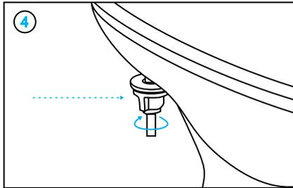
Tighten the bolts from below the toilet bowl until the seat is held securely.
