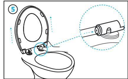
Once the seat is aligned and secured, press the quick release buttons and lift the seat upward to release it from the mounting bracket.
