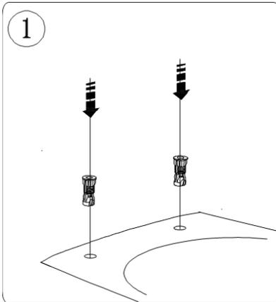
1) From above, insert and push expandable plastic anchors into seat fixing holes in bowl until they are flush with the surface.
