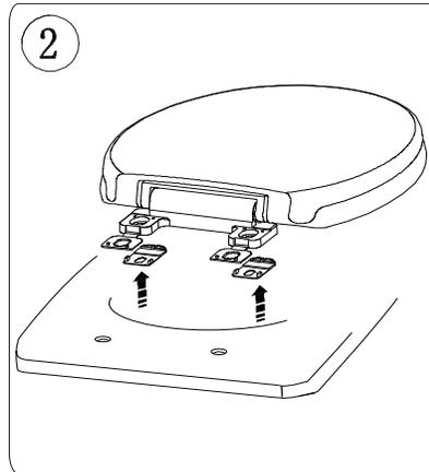
2) Insert rubber washers into the bottom of seat hinges.
