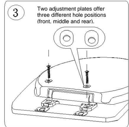
3) Fit seat onto the bowl. Choose the hole in the adjustment plate that best aligns with the seat fixing holes in the bowl. Put screws through holes and thread into expandable anchor without tightening.
