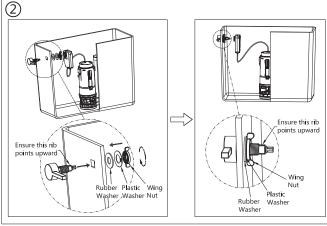
With the handle lever pointing towards the front of the tank, insert the handle assembly into the square hole in the tank wall. Place the black rubber washer and then the plastic washer over the handle assembly and then tighten the wing nut by hand.
