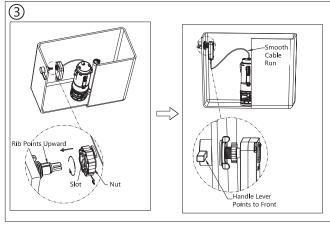
Connect the cable box to the side lever handle by aligning rib on the handle assembly with the slot on the cable box outer nut. Turning counter-clockwise, tighten the nut by hand or with a hand tool. NOTE: When attaching the cable box, ensure the cable does not interfere with the operation of the inlet valve.
