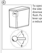
To operate, push the side lever downwards for a full flush. Pull the side lever upwards for a reduced flush.
