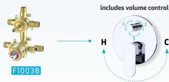
To turn the shower on and control water volume, pull the large handle outward. To regulate temperature, turn the large handle to the left for warmer water and to the right for cooler water. To divert water beween three shower elements, turn the smaller, diverter handle to align the indicator with the desired position.
