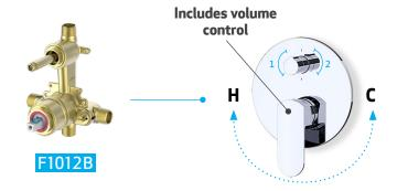
To turn the shower on and control water volume, simply pull the larger handle outward. To regulate the temperature, turn the large handle to the left for warmer water and to the right for cooler water. To divert water from one element to another, turn the smaller, diverter handle to the left or right. The water temperature does not have to be adjusted each time you divert the water between elements.
