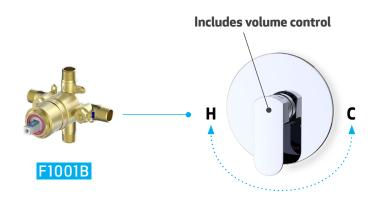
The F1001B is the height of straightforward efficiency. To turn water on and adjust volume to single shower element, pull the handle outward. To increase water temperature, turn the handle to the left and to decrease it, turn the handle to the right. Turn water off by pushing the handle back in to the starting position.
