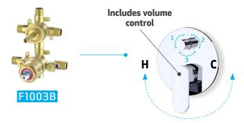
To turn the shower on and control water volume, pull the larger handle outward. To regulate temperature, turn the large handle to the left for warmer water and to the right for cooler water. To divert water beween three shower elements, turn the smaller, diverter handle in a circular motion, clicking between elements.
