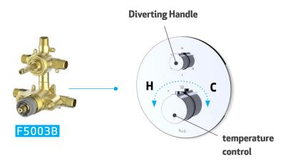
To turn water on to the desired shower element, turn the smaller, upper handle in a circular motion; in between each element position is a system 'off' position. To adjust water temperature, turn the lower, larger handle to the left for warmer water and to the right for cooler water. The valve automatically locks at a maximum temperature of 100 degrees. To exceed that temperature, push the safety button in and continue to turn to the left.
