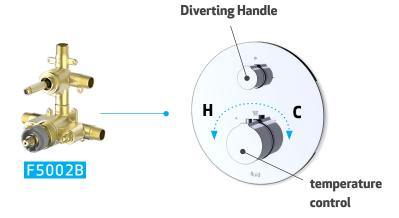
When the small, upper handle indicator is pointed upward, the system is off. To turn water on to a shower element, turn either left or right. To adjust water temperature, turn the lower, larger handle to the left for warmer water and to the right for cooler water. The valve automatically locks at a maximum temperature of 100 degrees. To exceed that temperature, push the safety button in and continue to turn to the left.
