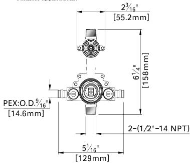
fluid Pressure Balancing Valve with 2 Way Diverter Model: F1012B-PEX-W
