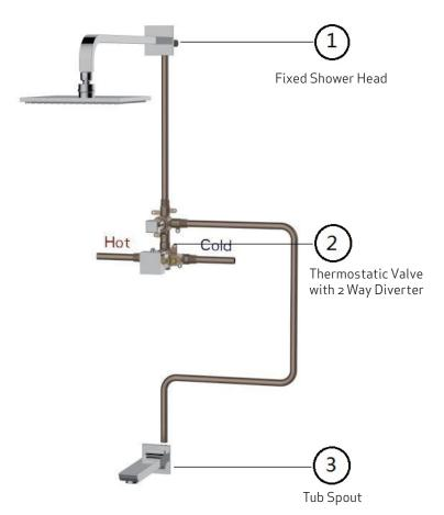
Water Flow For 2 Way Diverter Valve • Closed - Open
