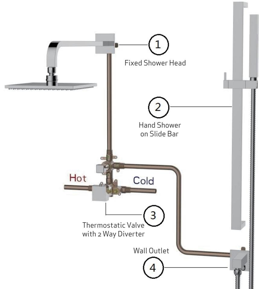
Water Flow For 2 Way Diverter Valve ○ Closed — Open
