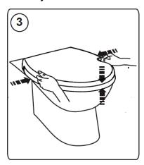
3) Now you are able to swivel the hinge into place to ensure proper seat alignment to howl
