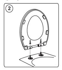
2) Insert hinge pins into the seat
