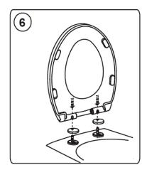
6) Cover the hinges on bowl with caps. Insert the seat back onto hinges. Your installation is now complete.
