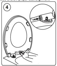
4) Once the seat is aligned well, lift the seat up and push the two quick release buttons on the inner center of seat underside to remove seat from the mounting bracket.
