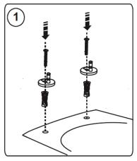
1) Fixing: From above, insert and push plastic anchors into seat fixing holes in bowl until they are flush with the surface. Tighten screws with a screw driver. Do not fasten screws too tightly; they must stay loose to allow proper seat alignment.
