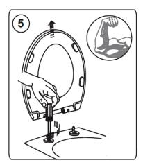
5) Tighten screws with a screw driver and cover the hinges on bowl with caps.
