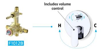
To turn the shower on and control water volume, simply pull the larger handle outward. To regulate the temperature, turn the large handle to the left for warmer water and to the right for cooler water. To divert water from one element to another, turn the smaller, diverter handle to the left or right. The water temperature does not have to be adjusted each time you divert the water between elements.
