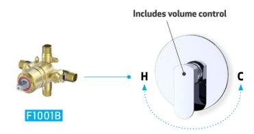
The F1001B is the height of straightforward efficiency. To turn water on and adjust volume to single shower element, pull the handle outward. To increase water temperature, turn the handle to the left and to decrease it, turn the handle to the right. Turn water off by pushing the handle back in to the starting position.
