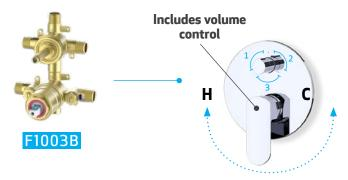
To turn the shower on and control water volume, pull the larger handle outward. To regulate temperature, turn the large handle to the left for warmer water and to the right for cooler water. To divert water beween three shower elements, turn the smaller, diverter handle in a circular motion, clicking between elements.
